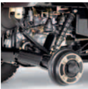
Strong leaf spring rear suspension with coil sprung dampers handles the heavy load capacity and ensures a smooth, stable ride over rugged terrain.
