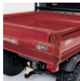
Tilting cargo bed with a 363 kg load capacity.
