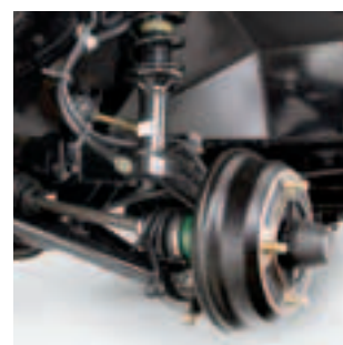
Independent front suspension allows each wheel to track over uneven ground for maximum traction with light steering effort.
