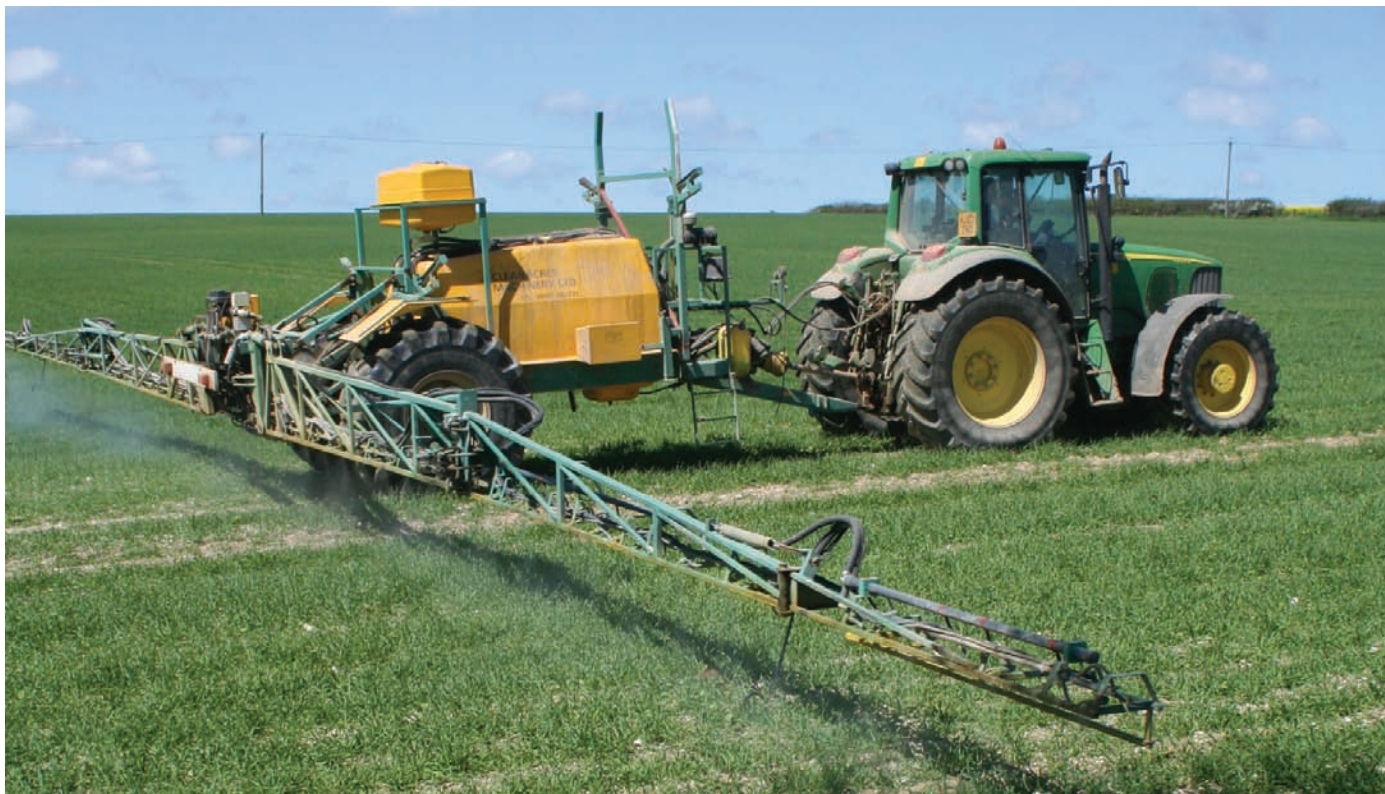
Twin fluid nozzles balance air and liquid pressure to produce a defined spray quality that gives good crop coverage and adherence, which helps pesticides do their job as effectively as possible.
