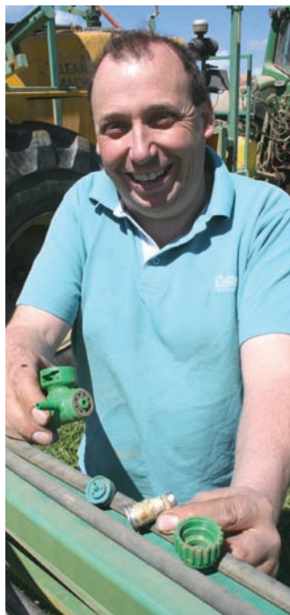
Spare Airtec nozzle – taken apart to show body, restrictor, anvil flood jet and cap – is rarely needed thanks to durable design and build.
